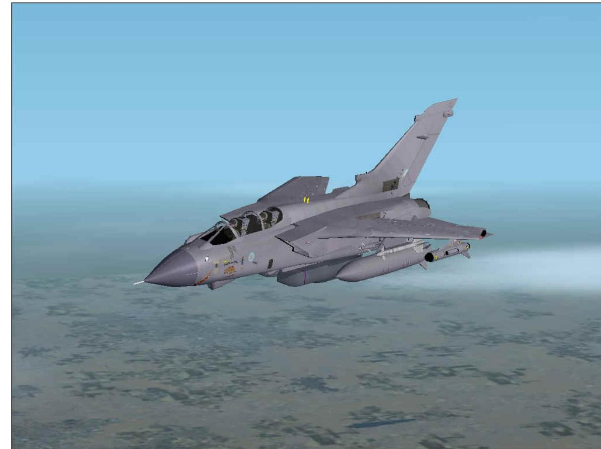
When the wings are swept back, the Tornado GR4 increases its high-speed low-level capability by reducing drag. When sweeping, the wings partially slide into the fuselage, reducing the exposed wing area. This gives the aircraft a low gust response in turbulent low-level winds. This not only makes flight much more comfortable for the aircrew but makes the aircraft a more stable platform from which to aim and deliver unguided weapons at low level.
