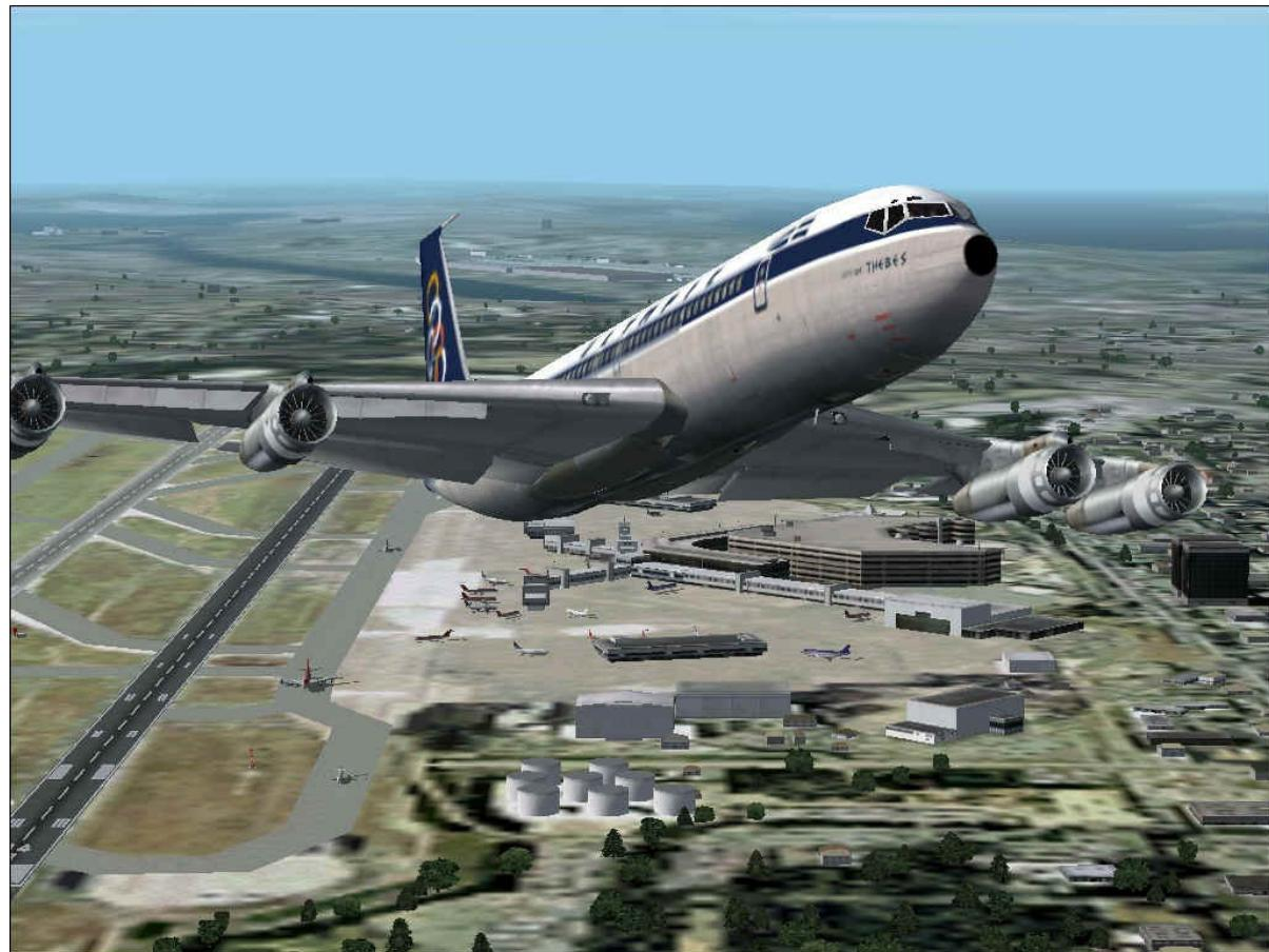
The 707’s engines could not supply sufficient bleed air for pressurization without a serious loss of thrust, so the aircraft instead used engine-driven turbocompressors to supply high-pressure air for this purpose. On many commercial 707s the outer port (#1) engine mount is distinctly different from the other three, as this is the only engine not fitted with a turbocompressor. The Boeing 707 was the first commercially successful airplane to use podded engines.
